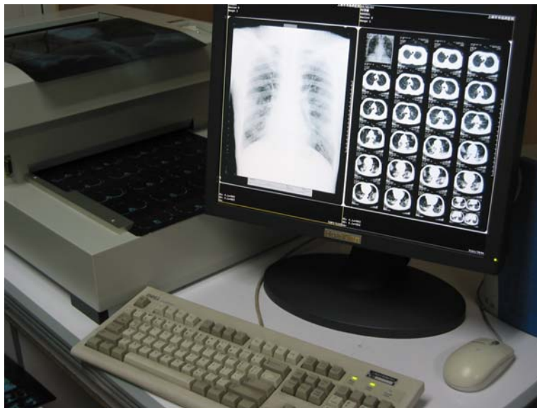
Figure 4. The film images of SARS patients were digitized by a laser digitizer for network delivering.
