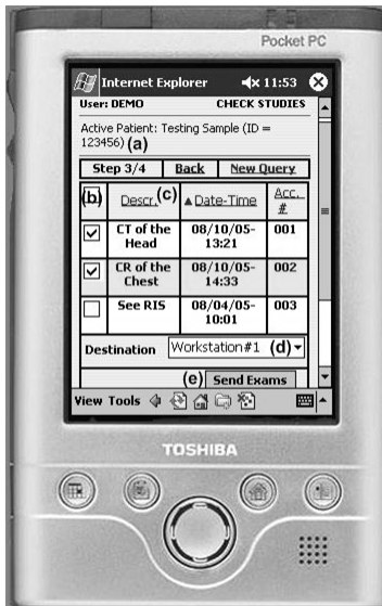
Figure 4 – Step 3: This screen shows the list of studies available for the selected patient. (a) displays the patient’s name and ID as reference to the user. The checkbox (b) allows the user to select all studies, or each study at the appropriate checkboxes. The user can also sort by Study Description, Study Date-Time, or Accession Number; all those columns are shown in (c). The user then selects where to send the selected examinations to by checking the “Destination” list (d). Finally, clicking the “Send Exams” button (e) completes the retrieval process.
